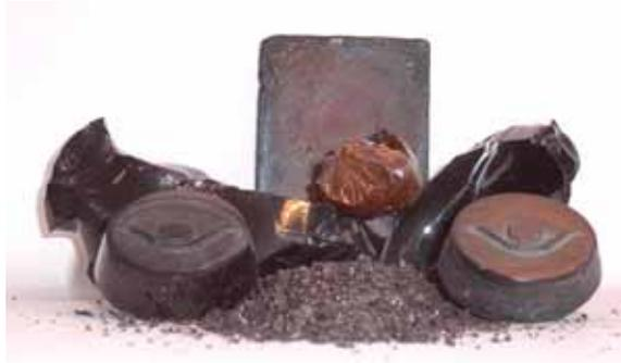
Fig. 3. Sample Products from Slag
