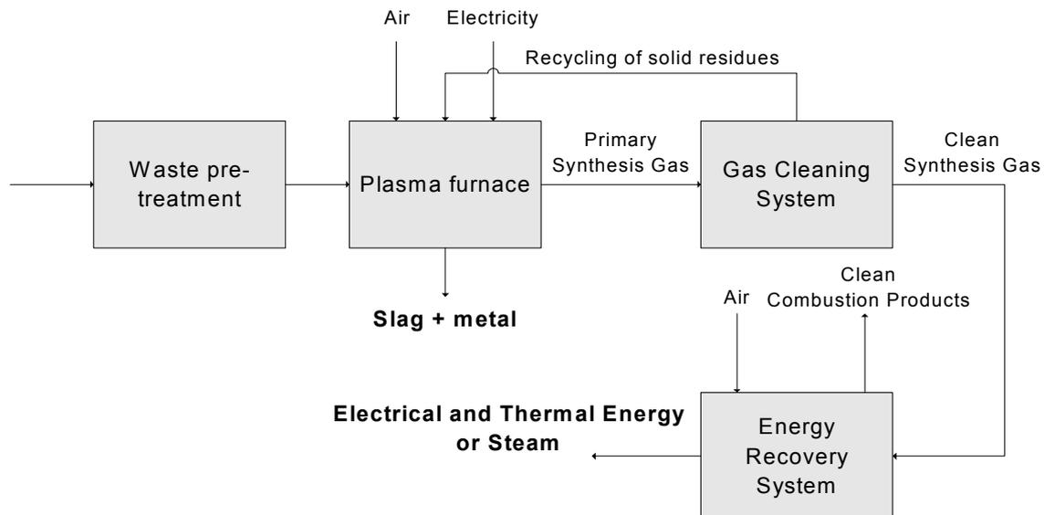
**Figure 1:** Block diagram of plasma waste treatment process
