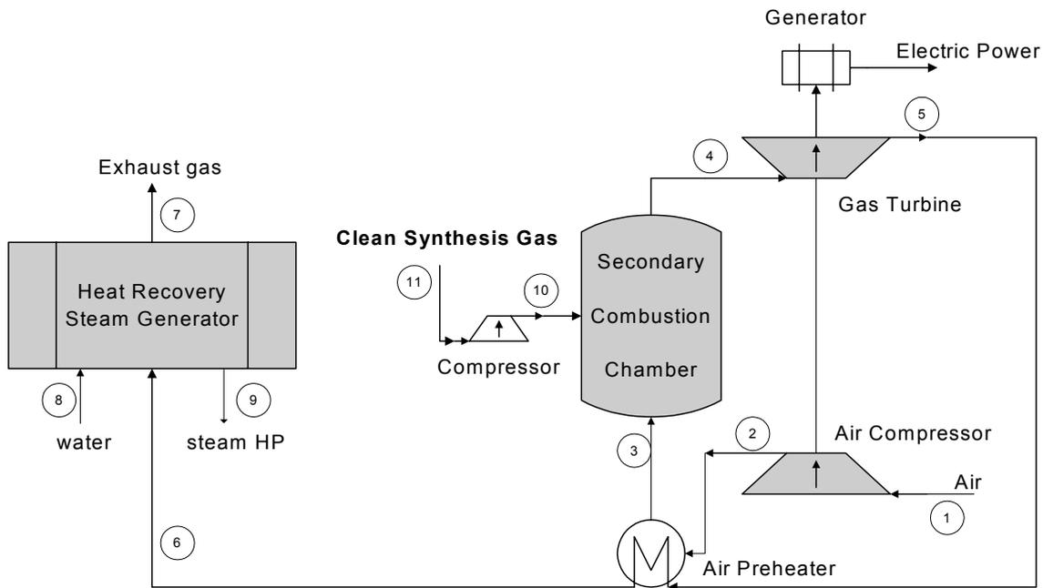
**Figure 2:** Energy recovery system – Cogeneration of steam and power
