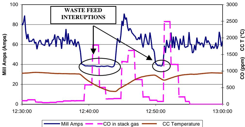
Fig. 5. Example of Data Acquisition During Inconsistent Feed Periods
