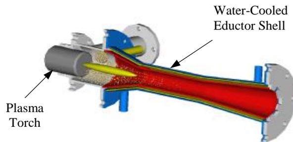
Fig. 2. Schematic of Plasma-Fired Eductor
