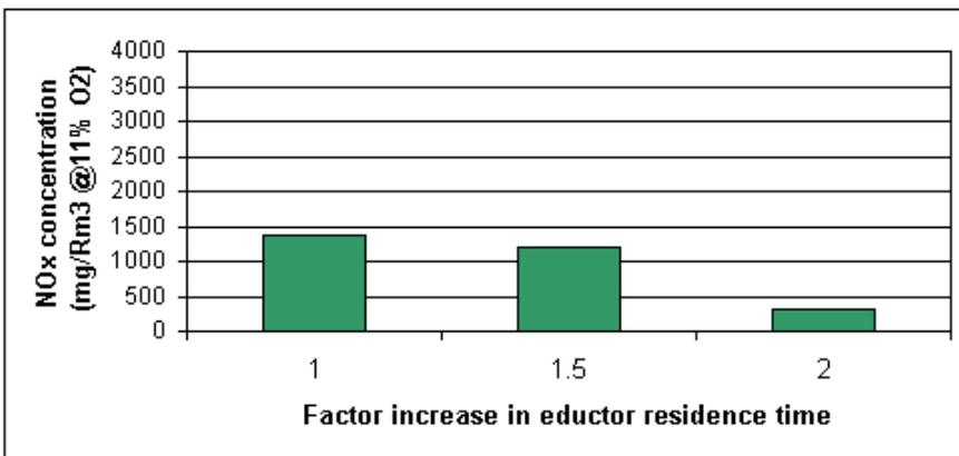
Fig. 9. Effect of Increasing Residence Time on NO<sub>x</sub> Emission
