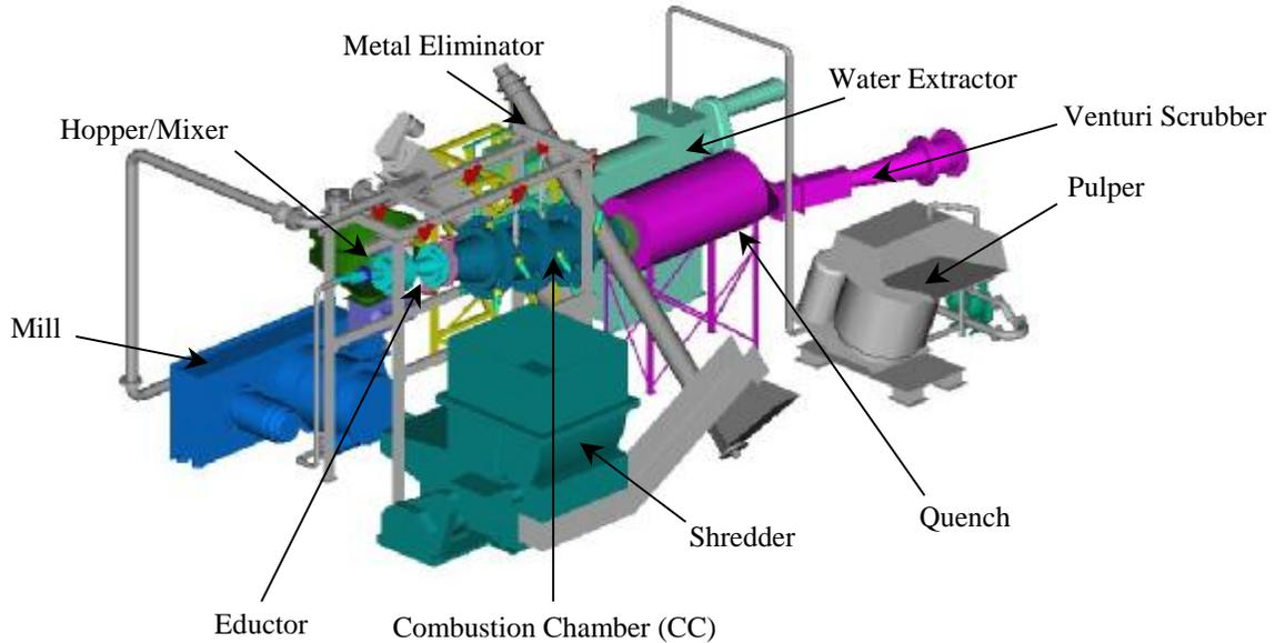
Fig. 1. Overall Layout Drawing of PAWDS
