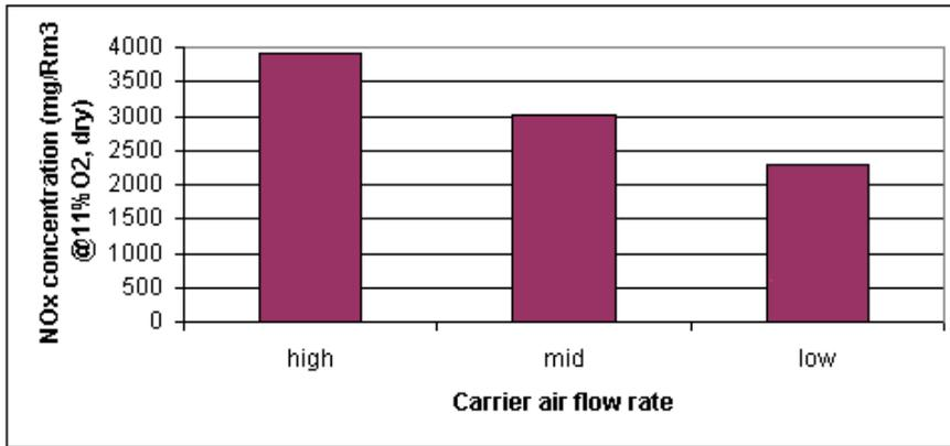
Fig. 7. Effect of Reducing Carrier Air Flow on NO<sub>x</sub> Emission
