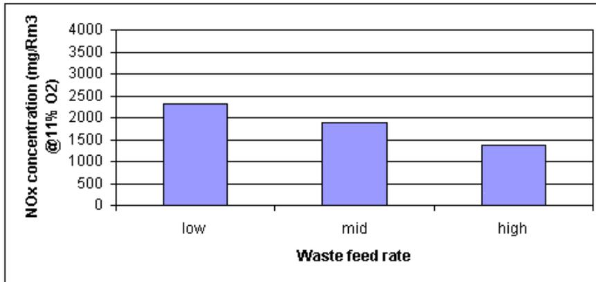
Fig. 8. Effect of Increasing Waste feed Rate on NO<sub>x</sub> Emission
